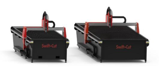
**XP 3000 (XP 510)** 3000mm x 1500mm cutting area (10' x 5') **4000 (XP 613)** 4000mm x 2000mm cutting area (13' x 6.5')
